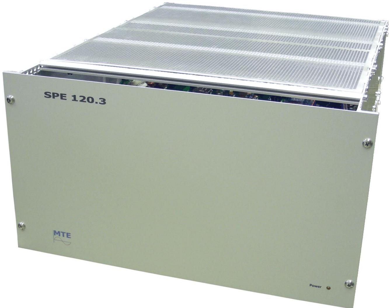
The SPE 120.3 is a three-phase computer controlled voltage and current source, designed for use in meter test systems and in the laboratory. It is in two performance steps with 300 VA and 600 VA output power available. The models are housed within a 19"-plug-in unit, 6 or 9 height modules, depending on output power.
